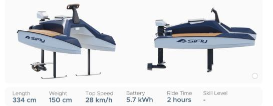
The Overboat is an electric catamaran that defies the traditional boating experience. Equipped with an electric propulsion system and multiple hydrofoils, it glides over the water, generating zero emissions, noise and wake. On the Overboat, anyone can easily and safely experience the unique sensation of flying over the waves.
